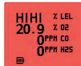
Red display in alarm conditions
