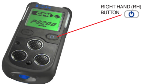
Fig. 2-1 PS200 Switch ON
