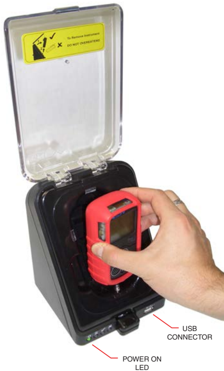
Fig. 6-2 Charging using Auto Bump / Calibration Station
