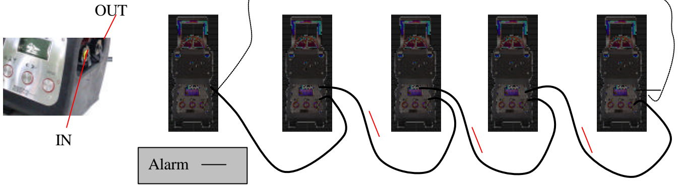
Staight forward alarm transfert
