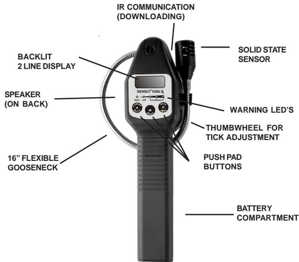
**Sensit® HXG-3** instruments are constructed of durable ABS plastic to withstand the rigors of field use.
