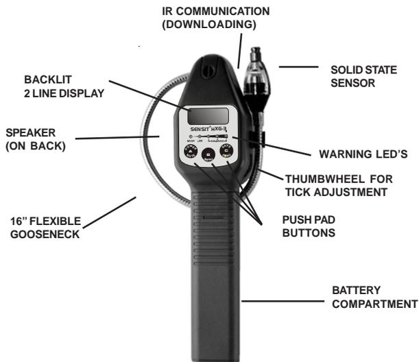
**Sensit® HXG-3P** instruments are constructed of durable ABS plastic to withstand the rigors of field use.
