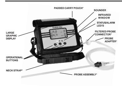
**TRAK-IT®IIIa** instruments are constructed of durable stainless steel to withstand the rigors of field use.
