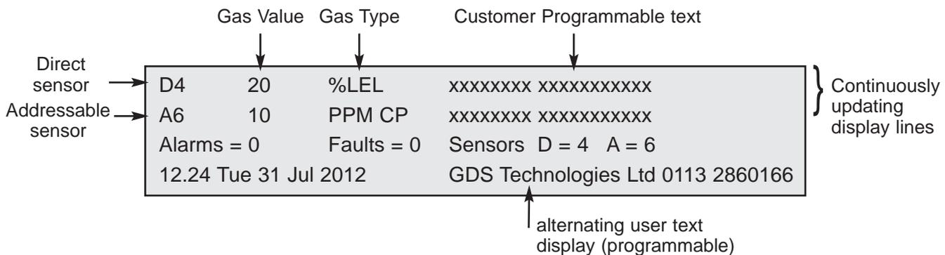
**Line 1** Standard 4~20mA sensor, values and gas type and location
