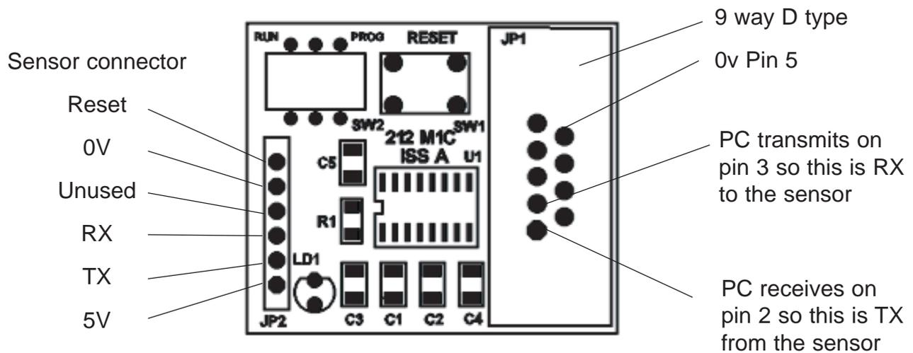
When programming the sensor processor, the Run and Prog slide switch SW2 is set to Prog but under normal circumstances, this switch should be in the Run position.
