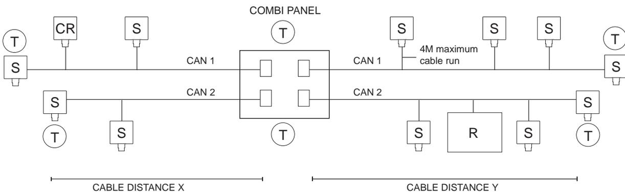
Maximum cable distance for CAN signal  $X+Y = 1\text{km}$
