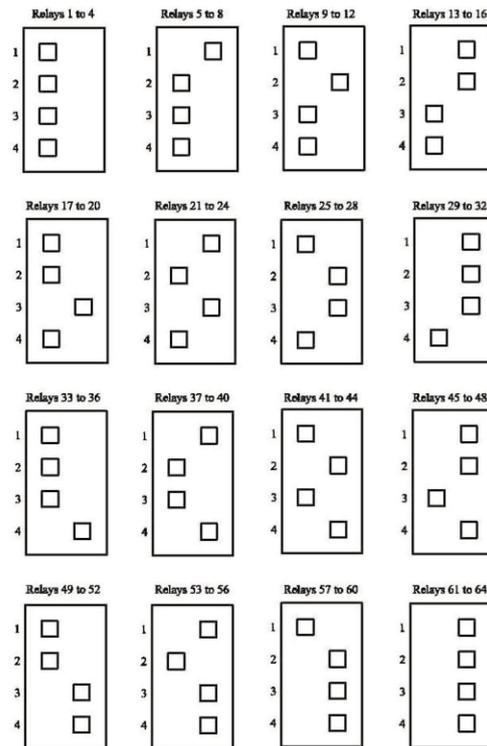
The eight channel 4~20mA output PCB allows signals in either sink or source mode to synchronised with the Combi 64 addressable and 16 direct sensors. By address selection on •S2Ž, the eight outputs can be selected for combinations of Combi sensors as detailed below.
