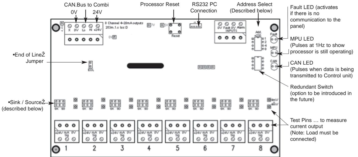
The Combi detects the address being used on this card when connected to the CAN-bus. According to the address, the outputs represent the following:
