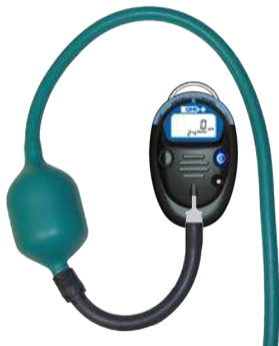
Fig. 2-12 Remote Sampling Set-up
