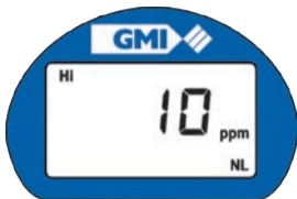
Fig. 2-4 Hi Alarm Level
