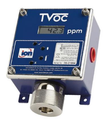
TVOC is a fixed photoionisation detector (PID) for the continuous measurement of total volatile organic compounds (VOCs). TVOC accurately measures over three different detection ranges from just one instrument.
