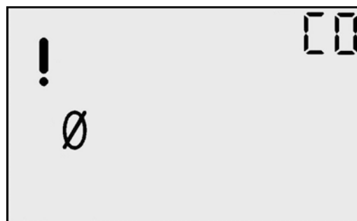
Zeroing Failed Screen
