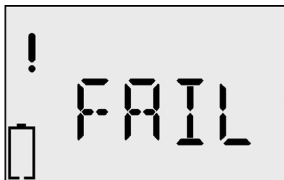
Battery Failure Screen
