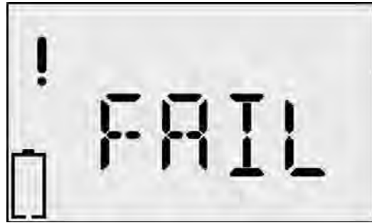
Battery Failure Screen
