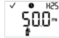
Bump test apply gas
