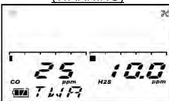
TWA Alarm Setpoint Display(*)
