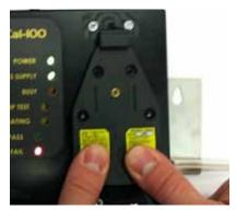
The BUMP and GAS LED's will illuminate indicating gas is being applied for the bump test.
